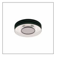
Lunis 11 R, downlight, light control with reflector, highly specular, light emission: direct distribution, LED rated luminous flux: 3.830lm, light colour: 930, with terminal, 3+2-pole, max. 2.5mm², mains connection: 230V, AC, 50/60Hz, black, diameter: 380mm, protection rating (complete): IP20, insulation class (complete): insulation class I (protective earthing), certification: CE, standard: EN 50419, packaging unit: 1 piece
