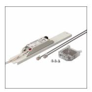
Monsun® 11/21, DALleco master kit, installation type: recessed, with cable with RJ-11 plug + 4x single conductor 0.75mm², AC, 50/60Hz, length: 250mm, width: 34mm, height: 29mm, DALleco controller, master, sensor HC1, light sensor deactivated, certification: CE, permissible operating ambient temperature: -25..+35°C, packaging unit: 1 piece
