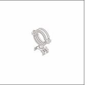
Monsun® 11/21, pipe clip fixing, installation type: surface-mounted, mounting set, consisting of each 2x pipe clamps of galvanised steel with rubber inlay, cylinder head screw, mounting clip for luminaire of V2A and 2x fixing reinforcement of UV-stabilised PC, clamping range: for pipe diameter 1.5", packaging unit: set of 2
