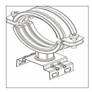
Monsun® 11/21, pipe clip fixing, installation type: surface-mounted, mounting set, consisting of each 2x pipe clamps of galvanised steel with rubber inlay, cylinder head screw, mounting clip for luminaire of V2A and 2x fixing reinforcement of UV-stabilised PC, clamping range: for pipe diameter 2", packaging unit: set of 2
