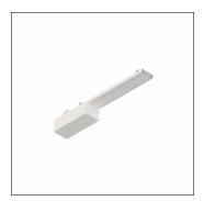
SITECO Connect IP Gen.1, rail insert, IP LAN connector, with plug, 6-pole, with phase selection, mains connection: 230V, AC, 50Hz, adapter, of sheet steel, coil coated, traffic white (RAL 9016), length: 450mm, width: 64mm, height: 38mm, protection rating (complete): IP40, insulation class (complete): insulation class I (protective earthing), certification: CE, UKCA, packaging unit: 1 piece
