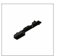
SITECO Connect IP Gen.1, rail insert, PoE universal adapter,with plug, 6-pole, with phase selection, mains connection: 230V, AC, 50Hz, adapter, of sheet steel, coil coated, jet black (RAL 9005), length: 500mm, width: 64mm, height: 65mm, protection rating (complete): IP40, insulation class (complete): insulation class I (protective earthing), certification: CE, UKCA, packaging unit: 1 piece
