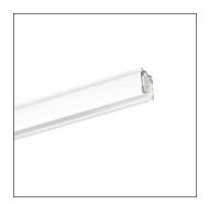
AX T, 3-phase track, installation type: suspended mounting, surface-mounted, control gear: ON/OFF, mains connection: 220..240V/380..400V, AC, of extruded aluminium section, coated, white, length: 2.000mm, width: 32mm, height: 33mm, protection rating (complete): IP20, insulation class (complete): insulation class I (protective earthing), certification: CE, ENEC, packaging unit: 1 piece
