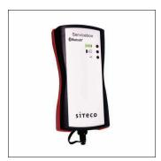
Street Light Control, Siteco® Service Box, control gear: DALI, control: digital communication interface, Bluetooth 4.0, with system connector: plug/socket, 4-pole, DC, housing, of plastic, dark grey, Siteco® Service Box, control via: Siteco Digital Interface, protection rating (complete): IP54, insulation class (complete): insulation class II (safety insulation), certification: CE, permissible operating ambient temperature for outdoor applications: 0..+50°C, packaging unit: 1 piece
