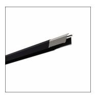
Licross®, trunking rail, of sheet steel, galvanised, coil coated, matt jet black (RAL 9005), length: 1.500 mm, width: 64 mm, height: 67mm, through-wiring: 9x 2.5mm², protection rating (complete): maximum IP64, depends on used inserts and accessories, insulation class (complete): insulation class I (protective earthing), certification: CE, UKCA, LABS conformity tested according to VDMA 24364:2018-05, packaging unit: 1 piece
