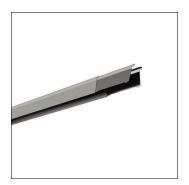
Licross®, trunking rail, of sheet steel, galvanised, coil coated, metallic grey (RAL 9006), length: 4.500 mm, width: 64 mm, height: 67mm, protection rating (complete): maximum IP64, depends on used inserts and accessories, insulation class (complete): insulation class I (protective earthing), certification: CE, UKCA, LABS conformity tested according to VDMA 24364:2018-05, packaging unit: 1 piece
