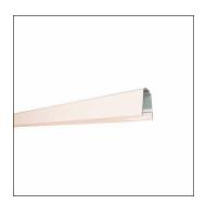
Licross®, mounting rail, of sheet steel, galvanised, coil coated, white, length: 2.250 mm, width: 64 mm, height: 67mm, protection rating (complete): maximum IP64, depends on used inserts and accessories, insulation class (complete): insulation class I (protective earthing), certification: CE, UKCA, LABS conformity tested according to VDMA 24364:2018-05, packaging unit: 1 piece
