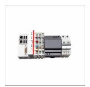
SITECO Connect 11base package S/D, 1..15 DALI lines, DIN rail PC, central control - connection to lighting or building management, installation type: recessed, installation location: in an electrical distributor, protection rating (complete): IP20, insulation class (complete): insulation class I (protective earthing), certification: CE, voltage: 230V, voltage type: AC, 1 x DALI-2, software: Lighting Solution, packaging unit: 1 piece
