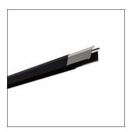
Licross®, trunking rail, of sheet steel, galvanised, coil coated, matt jet black (RAL 9005), length: 1.500 mm, width: 64 mm, height: 67mm, protection rating (complete): maximum IP64, depends on used inserts and accessories, insulation class (complete): insulation class I (protective earthing), certification: CE, UKCA, LABS conformity tested according to VDMA 24364:2018-05, packaging unit: 1 piece
