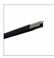
Licross<sup>®</sup>, trunking rail, of sheet steel, galvanised, coil coated, matt jet black (RAL 9005), length: 4.500 mm, width: 64 mm, height: 67mm, protection rating (complete): maximum IP64, depends on used inserts and accessories, insulation class (complete): insulation class I (protective earthing), certification: CE, UKCA, LABS conformity tested according to VDMA 24364:2018-05, packaging unit: 1 piece
