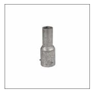
reducer, installation type: post-top, reducing sleeve, of St 37-2, galvanised, length: 230mm, diameter: 42mm, spigot size: 60/42mm, packaging unit: 1 piece
