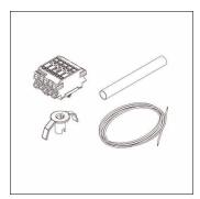
Monsun® 11/21, through-wiring, installation type: recessed, through-wiring set,5-core, 2.5mm², cable length: 1,7m, terminal,5-pole, max. 2.5mm², with protective earth, insulation class (complete): insulation class I (protective earthing), packaging unit: 1 piece
