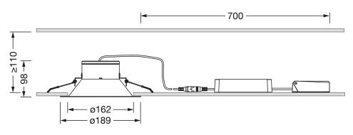
It is mandatory that the assembly instructions must be observed when planning and installing the electrical installation (to be found at www.siteco.com) Tolerances related to thermal, electrical and photometric data according to IEC 62722 Issued 16.02.2024 - Modifications and errors subject to change - Ensure that you always use the latest version -
