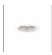
Lunis 31, midi, downlight, light control with lens, light emission: direct distribution, LED rated luminous flux: 2.150lm, light colour: 840, mains connection: 220..240V, AC, 50/60Hz, housing, white, protection rating (complete): IP20, protection rating (on room side): IP54, insulation class (complete): insulation class II (safety insulation), certification: CE, packaging unit: 1 piece
