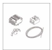
Monsun® 11/21, through-wiring, installation type: recessed, through-wiring set,7-core, 2.5mm², cable length: 1,4m, terminal,7-pole, max. 2.5mm² (5G+2), with protective earth, insulation class (complete): insulation class I (protective earthing), packaging unit: 1 piece
