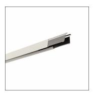
Licross®, trunking rail, of sheet steel, galvanised, coil coated, white, length: 3.000 mm, width: 64 mm, height: 67mm, through-wiring: 14x 2.5mm<sup>2</sup>, protection rating (complete): maximum IP64, depends on used inserts and accessories, insulation class (complete): insulation class I (protective earthing), certification: CE, UKCA, LABS conformity tested according to VDMA 24364:2018-05, packaging unit: 1 piece
