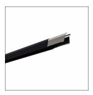
Licross®, trunking rail, of sheet steel, galvanised, coil coated, matt jet black (RAL 9005), length: 4.500 mm, width: 64 mm, height: 67mm, through-wiring: 7x 2.5mm², protection rating (complete): maximum IP64, depends on used inserts and accessories, insulation class (complete): insulation class I (protective earthing), certification: CE, UKCA, LABS conformity tested according to VDMA 24364:2018-05, packaging unit: 1 piece
