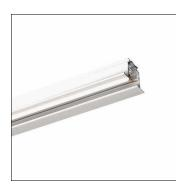
AX T, 3-phase track, installation type: recessed, control gear: DALI, mains connection: 220..240V/380..400V, AC, of extruded aluminium section, coated, white, length: 2.000mm, width: 32mm, height: 33mm, protection rating (complete): IP20, insulation class (complete): insulation class I (protective earthing), certification: CE, ENEC, packaging unit: 1 piece
