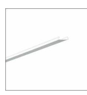
DUS<sup>®</sup> IP20DUS<sup>®</sup> mounting rail, blank cover, installation type: surface-mounted, blank cover, of plastic, uncoated, white, can be cut to suit, length: 1.535mm, width: 60mm, height: 20mm, protection rating (complete): IP20, packaging unit: 1 piece
