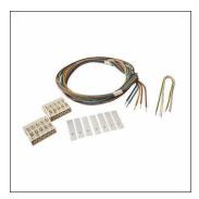
Monsun® 21 Gen.1, through-wiring, installation type: recessed, through-wiring set,5-core, 2.5mm², cable length: 1,4m, terminal,5-pole, max. 2.5mm², with protective earth, insulation class (complete): insulation class I (protective earthing), packaging unit: 1 piece
