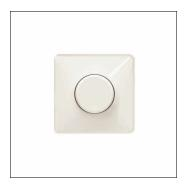
SITECO Connect 41 Rotaryrotary dimmer, master, local control - self-sufficient standalone sensors, dimmable, installation type: recessed, installation location: in the switch box, of plastic, protection rating (complete): IP20, insulation class (complete): insulation class II (safety insulation), certification: CE, voltage: 230V, voltage type: AC, 1 x rotary button/push button, 1 x DALI, packaging unit: 1 piece
