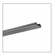
Vega® 11, mounting rail, installation type: suspended mounting, with terminal, 3+3-pole, max. 2.5mm², rail, of extruded aluminium section, anodised, natural, length: 4.000mm, width: 64mm, height: 22mm, protection rating (complete): IP20, certification: CE, packaging unit: 1 piece
