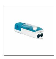
cable junction box, for 3 cables to 5x 16mm<sup>2</sup>, L1/L2/L3/N/PE, 1x E14, cable junction box, of plastic, shock-resistant, inner mast diameter: from 84mm, protection rating (complete): IP44, insulation class (complete): insulation class II (safety insulation), certification: CE, packaging unit: 1 piece
