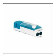
cable junction box, for 3 cables to 5x 16mm², L1/L2/L3/N/PE, 2x E14, cable junction box, of plastic, shock-resistant, inner mast diameter: from 84mm, protection rating (complete): IP44, insulation class (complete): insulation class II (safety insulation), certification: CE, packaging unit: 1 piece
