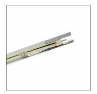
Modario®, trunking rail, of sheet steel, coated, pure white, 2-length, length: 2.392 mm, width: 58 mm, height: 43mm, through-wiring: 10x 2.5mm², with terminal, 10-pole, max. 2.5mm², protection rating (complete): for IP20/IP40 protection rating, insulation class (complete): insulation class I (protective earthing), certification: CE, ENEC, VDE, standard: EN 60598, packaging unit: 1
