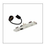
Modario<sup>®</sup>, rail insert, socket outlet, with plug, 3-pole, with phase selection, mains connection: 240V, AC, 50Hz, socket outlet insert, of sheet steel, coil coated, pure white, 1x system unit, length: 299mm, width: 48mm, protection rating (complete): for IP20 protection rating, insulation class (complete): insulation class I (protective earthing), certification: CE, packaging unit: 1 piece
