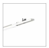
Modario®, track adapter insert, with plug, 5-pole, with phase selection, for trunking rail, 10-core, mains connection: 230/400V, track adapter insert, of sheet steel, coil coated, pure white, 2x system unit, max. weight load 5kg, length: 598mm, width: 48mm, protection rating (complete): for IP20 protection rating, insulation class (complete): insulation class I (protective earthing), certification: CE, packaging unit: 1 piece
