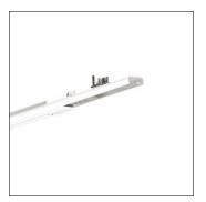
Modario®, track adapter insert, control gear: DALI, with plug, 5-pole, with phase selection, for trunking rail, 10-core, mains connection: 230/400V, track adapter insert, of sheet steel, coil coated, pure white, 4x system unit, max. weight load 5kg, length: 1.196mm, width: 48mm, protection rating (complete): for IP20 protection rating, insulation class (complete): insulation class I (protective earthing), certification: CE, packaging unit: 1 piece
