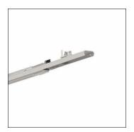
Modario®, track adapter insert, with plug, 5-pole, with phase selection, for trunking rail, 5 or 10-core, mains connection: 230/400V, track adapter insert, of sheet steel, coil coated, metallic grey (RAL 9006), 2x system unit, max. weight load 5kg, length: 598mm, width: 48mm, protection rating (complete): for IP20 protection rating, insulation class (complete): insulation class I (protective earthing), certification: CE, packaging unit: 1 piece
