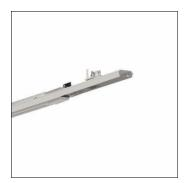
Modario®, track adapter insert, with plug, 5-pole, with phase selection, for trunking rail, 10-core, mains connection: 230/400V, track adapter insert, of sheet steel, coil coated, metallic grey (RAL 9006), 2x system unit, max. weight load 5kg, length: 598mm, width: 48mm, protection rating (complete): for IP20 protection rating, insulation class (complete): insulation class I (protective earthing), certification: CE, packaging unit: 1 piece
