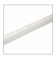
Modario<sup>®</sup>, additional feed, wiring, with 20x 2-fold terminal 1.5..2.5mm<sup>2</sup>, for infeed, through-wiring: 10x 2.5mm<sup>2</sup>, trunking rail element, of steel, coated, pure white, 4x system unit, length: 1.196mm, width: 58mm, height: 43mm, insulation class (complete): insulation class I (protective earthing), certification: CE, UKCA, packaging unit: 1 piece
