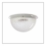
electrics components group, for Large Bell, control gear: ECG Plus, LED luminous flux: 3.210 lm, colour temperature: 3000K, mains connection: 230..240V, AC, 50/60Hz, start of lifetime: 23 W, end of service life: 24 W, reduction: 12 W, primary light characteristic: asymmetric, primary optical cover: enclosure, of PMMA, transparent structured, gear tray with cover, insulation class (complete): insulation class II (safety insulation), certification: CE, ENEC, VDE
