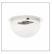
electrics components group, for Large Bell, control gear: ECG Plus, LED luminous flux: 3.320 lm, colour temperature: 4000K, mains connection: 230..240V, AC, 50/60Hz, start of lifetime: 23 W, end of service life: 24 W, reduction: 12 W, primary light characteristic: asymmetric, primary optical cover: enclosure, of PMMA, transparent, gear tray with cover, insulation class (complete): insulation class II (safety insulation), certification: CE, ENEC, VDE
