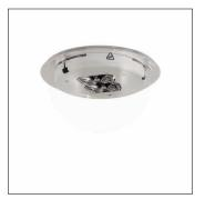
electrics components group, for Small Bell, control gear: ECG Plus, LED luminous flux: 1.640 lm, colour temperature: 3000K, mains connection: 230..240V, AC, 50/60Hz, start of lifetime: 13 W, end of service life: 14 W, reduction: 7 W, primary light characteristic: asymmetric, primary optical cover: enclosure, of PMMA, transparent, gear tray with cover, insulation class (complete): insulation class II (safety insulation), certification: CE, ENEC, VDE
