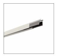
Licross®, trunking rail, of sheet steel, galvanised, coil coated, white, length: 1.500 mm, width: 64 mm, height: 67mm, through-wiring: 11x 2.5mm<sup>2</sup>, protection rating (complete): maximum IP64, depends on used inserts and accessories, insulation class (complete): insulation class I (protective earthing), certification: CE, UKCA, LABS conformity tested according to VDMA 24364:2018-05, packaging unit: 1 piece
