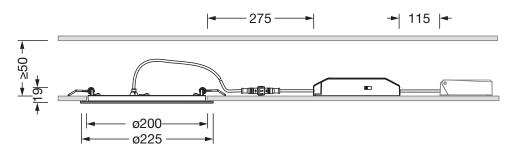
It is mandatory that the assembly instructions must be observed when planning and installing the electrical installation (to be found at www.siteco.com) Tolerances related to thermal, electrical and photometric data according to IEC 62722 Issued 15.03.2024 - Modifications and errors subject to change - Ensure that you always use the latest version -
