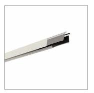
Licross®, trunking rail, of sheet steel, galvanised, coil coated, white, length: 3.000 mm, width: 64 mm, height: 67mm, through-wiring: 9x 2.5mm<sup>2</sup>, protection rating (complete): maximum IP64, depends on used inserts and accessories, insulation class (complete): insulation class I (protective earthing), certification: CE, UKCA, LABS conformity tested according to VDMA 24364:2018-05, packaging unit: 1 piece
