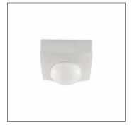
SITECO ConnectSensor-Head PR1-S, slave, local control - self-sufficient standalone sensors, central control - connection to lighting or building management, dimmable, installation type: slip-in mounting, installation location: on interface, of plastic, certification: CE, VDE, 1 x PIR movement sensor, 1 x light sensor, packaging unit: 1 piece
