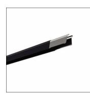
Licross<sup>®</sup>, trunking rail, of sheet steel, galvanised, coil coated, matt jet black (RAL 9005), length: 3.000 mm, width: 64 mm, height: 67mm, through-wiring: 9x 2.5mm<sup>2</sup>, protection rating (complete): maximum IP64, depends on used inserts and accessories, insulation class (complete): insulation class I (protective earthing), certification: CE, UKCA, LABS conformity tested according to VDMA 24364:2018-05, packaging unit: 1 piece
