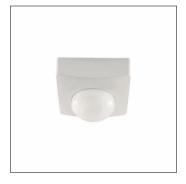
SITECO ConnectSensor-Head PC5-M, master, local control - self-sufficient standalone sensors, switchable, dimmable, installation type: slip-in mounting, installation location: on interface, of plastic, protection rating (complete): IP54, certification: CE, VDE, 1 x PIR movement sensor, 1 x light sensor, 1 x IR receiver, packaging unit: 1 piece
