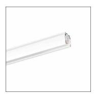
AX T, 3-phase track, installation type: suspended mounting, surface-mounted, control gear: DALI, mains connection: 220..240V/380..400V, AC, of extruded aluminium section, coated, white, length: 1.000mm, width: 32mm, height: 33mm, protection rating (complete): IP20, insulation class (complete): insulation class I (protective earthing), certification: CE, ENEC, packaging unit: 1 piece
