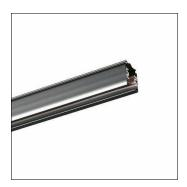
AX T, 3-phase track, installation type: suspended mounting, surface-mounted, control gear: DALI, mains connection: 220..240V/380..400V, AC, of extruded aluminium section, coated, jet black (RAL 9005), length: 3.000mm, width: 32mm, height: 33mm, protection rating (complete): IP20, insulation class (complete): insulation class I (protective earthing), certification: CE, ENEC, packaging unit: 1 piece
