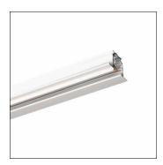
AX T, 3-phase track, installation type: recessed, control gear: ON/OFF, mains connection: 220..240V/380..400V, AC, of extruded aluminium section, coated, white, length: 2.000mm, width: 32mm, height: 33mm, protection rating (complete): IP20, insulation class (complete): insulation class I (protective earthing), certification: CE, ENEC, packaging unit: 1 piece
