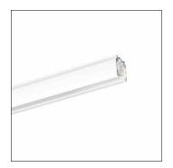
AX T, 3-phase track, installation type: suspended mounting, surface-mounted, control gear: DALI, mains connection: 220..240V/380..400V, AC, of extruded aluminium section, coated, white, length: 3.000mm, width: 32mm, height: 33mm, protection rating (complete): IP20, insulation class (complete): insulation class I (protective earthing), certification: CE, ENEC, packaging unit: 1 piece
