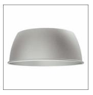
Highbay 31 L, reflector, primary light control with reflector, of aluminium, Alu-Soft, light emission: direct distribution, primary light characteristic: rotationally symmetric, installation type: surface-mounted, diameter: 590mm, height: 250mm, packaging unit: 1 piece
