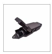
SITECO Connect Wirelesscontroller, lighting management components, master, local control - self-sufficient standalone sensors, dimmable, installation type: lay-in mounting, installation location: in the ceiling, voltage: 230V, 1 x DALI, 1 x Bluetooth<sup>®</sup> interface, 1 x switching contact, protection rating (complete): IP20, insulation class (complete): insulation class II (safety insulation), certification: CE, packaging unit: 1 piece
